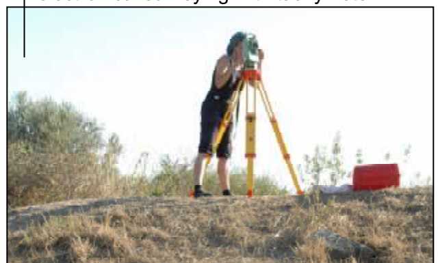
electronical surveying with tachymeter
