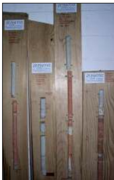
drilling cores and their positions (federal state authority for monuments, Prof. Snethlage)
