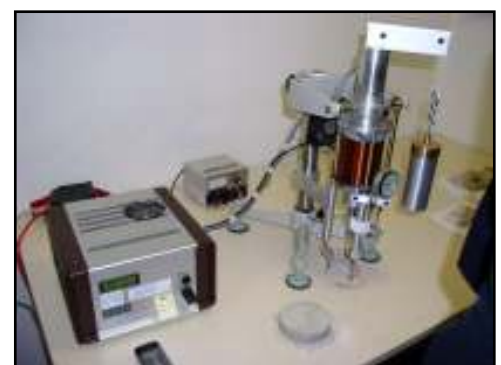
pressure testing of stone supplement material (Dr. Wendler, München)
